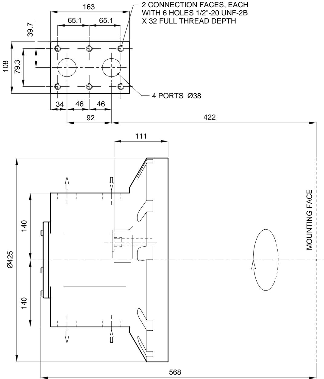
REVERSE PORT CONNECTIONS FOR OPPOSITE DIRECTION OF SHAFT ROTATION
