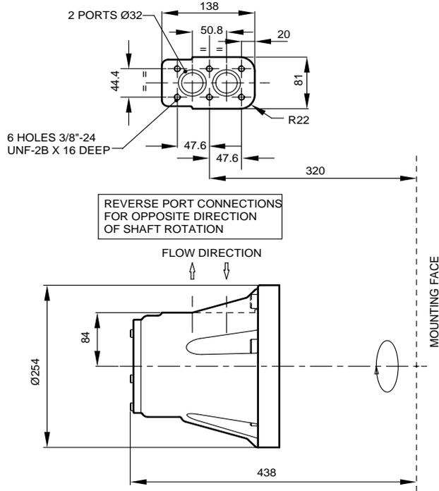
**2 1/4" Valve Housing with 1" SAE 4-Bolt Flanges, F2/'FM2'**
