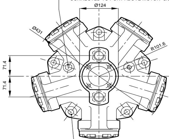
5 HOLES Ø18 EQUI-SPACED AS SHOWN ON A [305] P.C.D. SPOTFACED TO Ø38.
