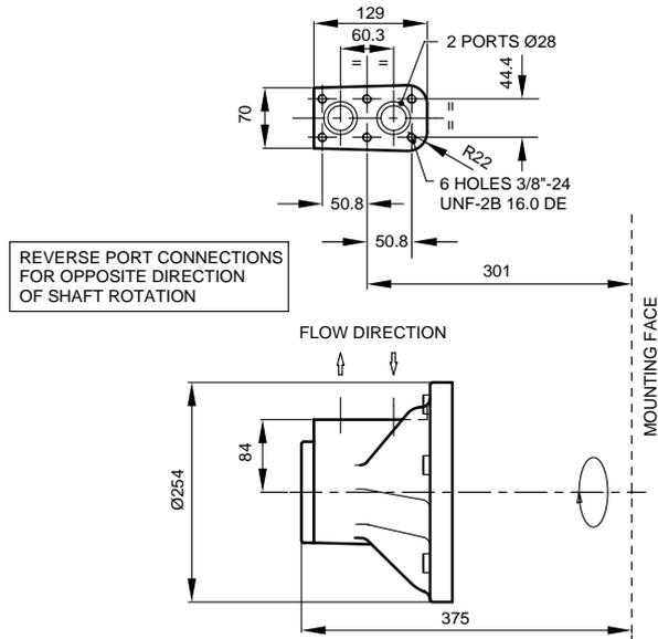
**4" VALVE HOUSING WITH 1 1/2" SAE 4-BOLT FLANGES, 'F4'/FM4'**
