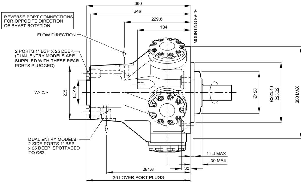
DRAIN CONNECTION 3/8 BSP x 19 DEEP SPOTFACED TO Ø28. CHOICE OF TWO POSITIONS ONE NORMALLY PLUGGED. ON INSTALLATION ENSURE DRAIN IS CONNECTED TO PORT ABOVE MOTOR C/L
