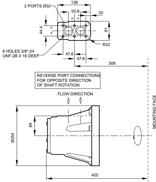
**2 1/4" VALVE HOUSING WITH 1" SAE 4-BOLT FLANGES,
