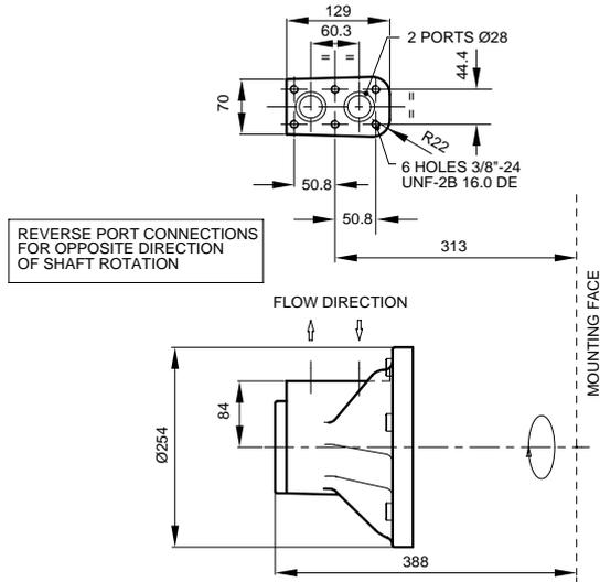
3" VALVE HOUSING WITH 1 1/4" SAE 4-BOLT FLANGES, 'F3'/FM3'
