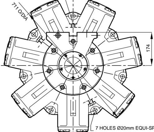
7 HOLES Ø20mm EQUI-SPACED AS SHOWN ON A[520.7] P.C.DIA.
