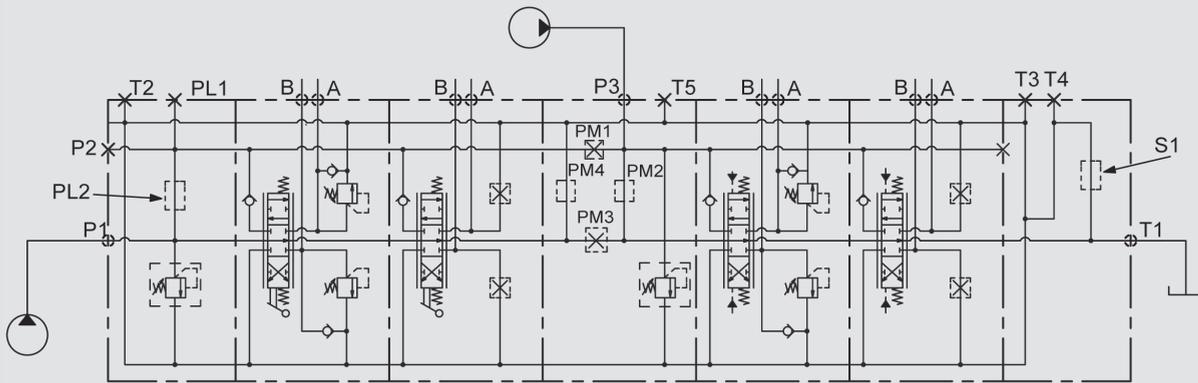
**Diagram 2: Two pump circuit with intermediate section (K3)**
