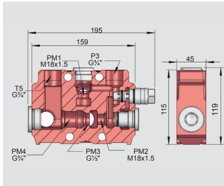
The intermediate section allows a number of different internal and external system alternatives.
