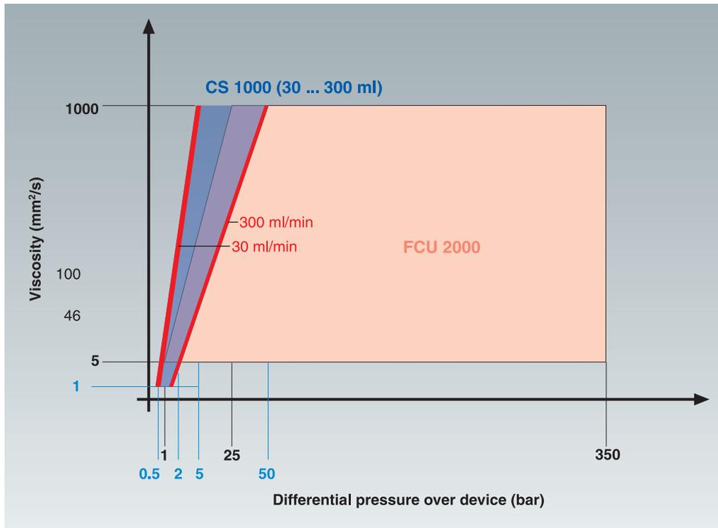
Various ConditioningModules (CM) are available for regulating the flow rate within the permissible range. The ConditioningModules enable the working range of the CS 1000 and CS 2000 to be adapted to the hydraulic conditions. These units are presented in a number of typical installation examples.
