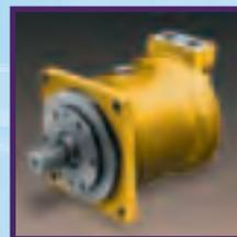
Multiple **M3X Series** axial piston hydraulic motors provide the driving force to turn a giant boring machine efficiently. A special spherical surface type valve plate significantly improves the starting efficiency, enabling the motor to start the machine under full load.
