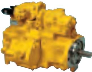
K7V pumps are high pressure open circuit axial piston pumps specially designed with shortened length for compact machine installation requirements.
