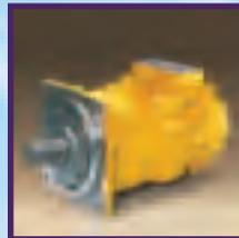
Connected directly to the ports of the hydraulic motors, the **KDC Series** counterbalance valve prevents loads from dropping freely and regulates lowering speed smoothly by generating the required back pressure to the winch motor.
