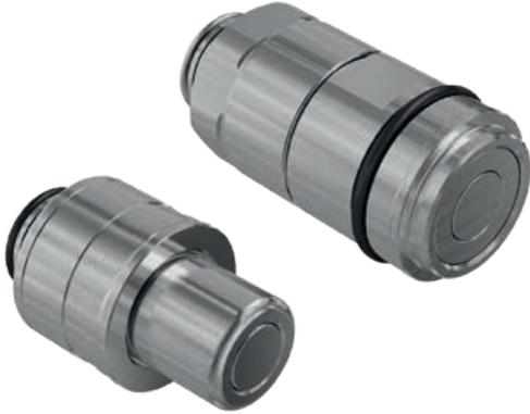
Flat Face Male and Female cartridge couplings in Stainless Steel (AISI 316) with Viton seals. Self-aligning couplings for MultiFaster. Misalignments up to  $\pm 0.5$  mm and  $\pm 1^\circ$  (angular) are automatically compensated during the connection. Available sizes: 1/4", 3/8", 1/2". Faster proprietary profile.
