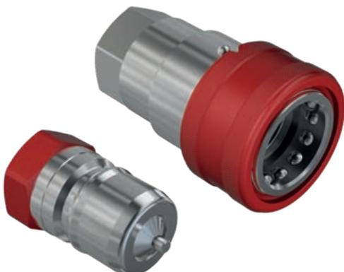
Male and Female couplings with poppet valve shut-off system, Lloyd's certified, suitable for Oil & Gas applications. Thanks to special components and seals, HNVFR couplings are API 16 D certified and suitable for BOP application. Available sizes: 1/2", 3/4", 1". Interchangeable according to ISO 7241 Part B.
