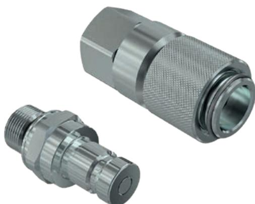
Diagnostic Flat Face Male and Female couplings, specifically designed to measure the internal pressure of hydraulic circuits. Male part to be mounted on the hydraulic line, Female part to be connected to gauge instruments. Available in size 1/4". Interchangeable according to ISO 15171-1.
