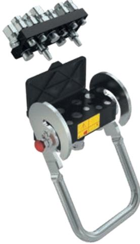
MultiFaster 10 lines. 5 lines size o8, 5 lines size o4. Working Pressure 25 MPa. Flow rate @ 0.2 MPa: 5 lines 70 l/min, 5 lines 20 l/min.
