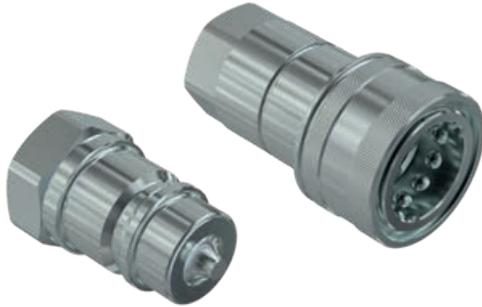
Male and Female couplings with poppet valve shut-off system. Size 1/2" interchangeable according to ISO 7241 Part A. Flow rate @ 0.2 MPa: 75 l/min.
