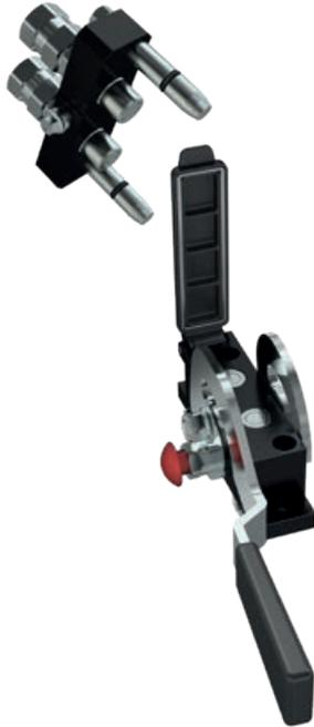
MultiFaster, 2 lines, size o6. Very compact design and dimensions. Working pressure: 25 MPa. Flow rate @ 0.2 MPa: 40 l/min.
