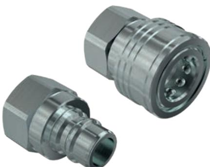
Male and Female couplings, suitable for Oil & Gas applications. Free Flow couplings. Designed to maximize flow, assembled without internal valves. Available sizes: 1/4", 1/2", 3/4". Interchangeable with Faster TNV couplings. Available also in brass (sizes 1", 1-1/2").
