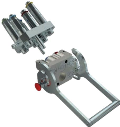
MultiFaster 5 lines. 2 lines size o6, 3 lines size o9, 1 housing for electrical connector. Working pressure 25 MPa. Flow rate @ 0.2 MPa: 2 lines 20 l/min, 3 lines 35 l/min.
