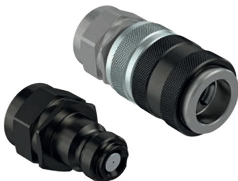
Male and Female couplings for Ultra High Pressure applications. Working pressures of 150 MPa. Very robust and reliable, equipped with safety sleeve. Characterized by redundant visual and mechanical safety systems. Available in size 1/4". Black caps provided as standard with the couplings.
