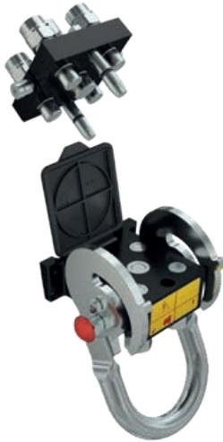
MultiFaster 5 lines. 4 lines o6 and 1 line o8. Line o8 can be replaced by an electrical connector. Working Pressure: 25 MPa. Flow rate @ 0.2 MPa: 4 lines 40 l/min, 1 line 70 l/min.
