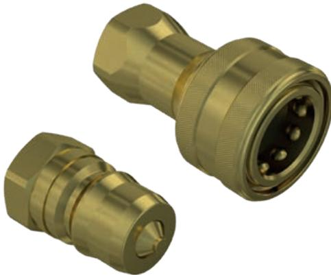
Male and Female couplings for industrial applications with poppet valve shut-off system. Brass version available with NBR or Viton seals. Available sizes: 1/8", 1/4", 3/8", 1/2", 3/4", 1", 1-1/2". Interchangeable according to ISO 7241 Part B.
