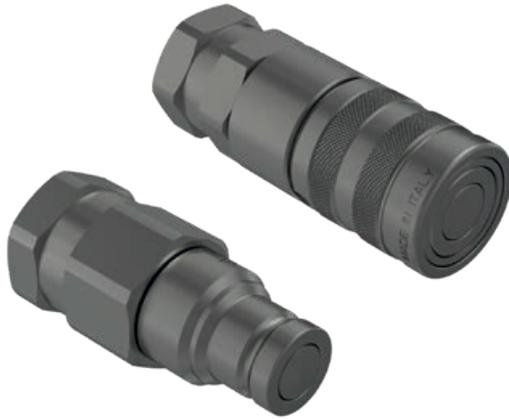
Flat face Male and Female couplings. The flat valve shut-off system prevents contamination and spillage. Real maximum working pressure of 35 MPa and Zinc-Nickel plating. Available sizes: 1/8", 1/4", 3/8", 1/2", 5/8", 3/4", 1". Interchangeable according to ISO 16028. Size 1/8" has surface treatment in Mate 500 (CrIII) and it is not ISO interchangeable.
