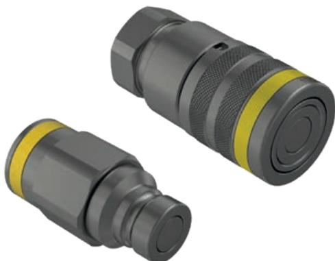
Flat Face Male and Female couplings, suitable for High Pressure applications. Flat valve shut-off system prevents contamination and spillage. Zinc-Nickel plating ensures good resistance to wear and corrosion. Maximum Working Pressure: 72 MPa. Available sizes: 1/4", 3/8".
