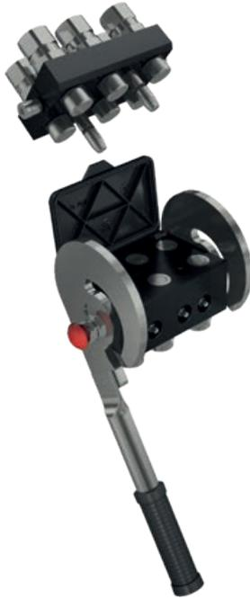
MultiFaster 6 lines, size o8, "G" type, with greaser and Zinc-Nickel plating. Working pressure: 25 MPa. Flow rate @ 0.2 MPa: 70 l/min.
