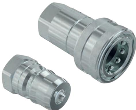
Male and Female couplings for industrial applications with poppet valve shut-off system. Stainless Steel version (AISI 316) with Viton seals. Available sizes: 1/4", 3/8", 1/2", 3/4", 1", 1-1/2", 2". Interchangeable according to ISO 7241 Part B.
