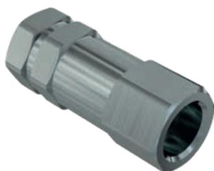
Standard unidirectional check valves, acting as a safety device into hydraulic systems. Standard versions contain a spring set to open the valve at 35 kPa; Normally available with inlet and outlet Female threads. Available sizes: 1/4", 3/8", 1/2", 3/4", 1", 1-1/4", 1-1/2", 2". Wide range of calibrations available, from 10 to 950 kPa.
