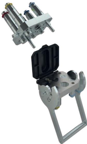
MultiFaster 5 lines. 3 lines size o6, 2 lines size o9, 1 housing for electrical connector. Working pressure 22 MPa. Flow rate @ 0.2 MPa: 3 lines 20 l/min, 2 lines 35 l/min.
