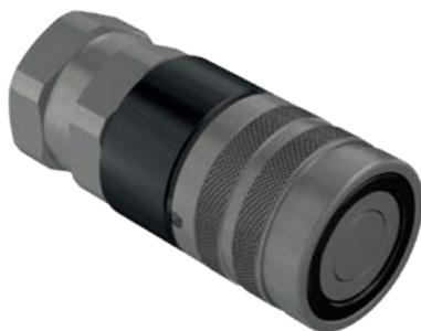
Flat face Female couplings, equipped with sector latching technology. The sector latching system enables to effectively tackle the Brinelling effect, provoked by high frequency impulse pressures.
