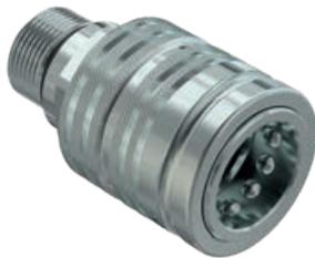
Female couplings designed for panel mounting installation and connection to flexible hoses. Wide range of threaded adapters available. Size 1/2". Interchangeable according to ISO 7241 Part A. Flow rate @ 0.2 MPa: 75 l/min.
