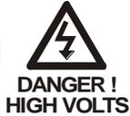
**WARNING: DANGER OF INJURY OR DEATH.** During normal operation, Sentinel is connected to high voltage AC circuits. Before connection, disconnection or handling of these chargers, ensure isolation of all AC power supplies. Connection or disconnection with live wiring can also cause hazardous sparking and component damage.
