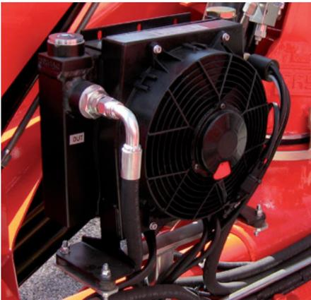
**Hydraulic oil cooling on loader crane:**
