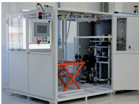
Thermal shock test rig
