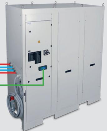
Separate auxiliary coolers with high capacities up to 160 kW for cooling tasks in the machine tool sector. Several units can be connected in parallel to expand the capacity as required.
