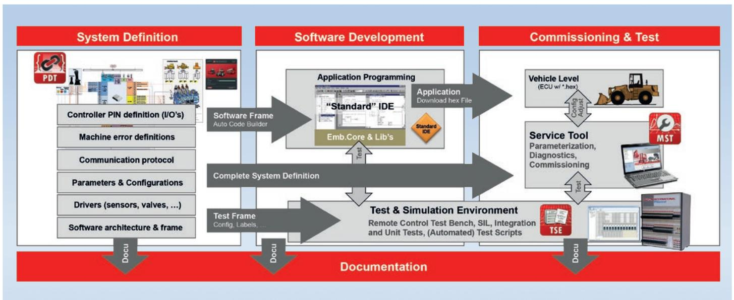
Since the system has been precisely co-ordinated using tools optimized for the individual tasks, interface losses and multiple inputs are almost completely avoided. All system parts have interfaces to enable documentation to be generated automatically. The enormous expense for documentation can be significantly reduced in this way.
