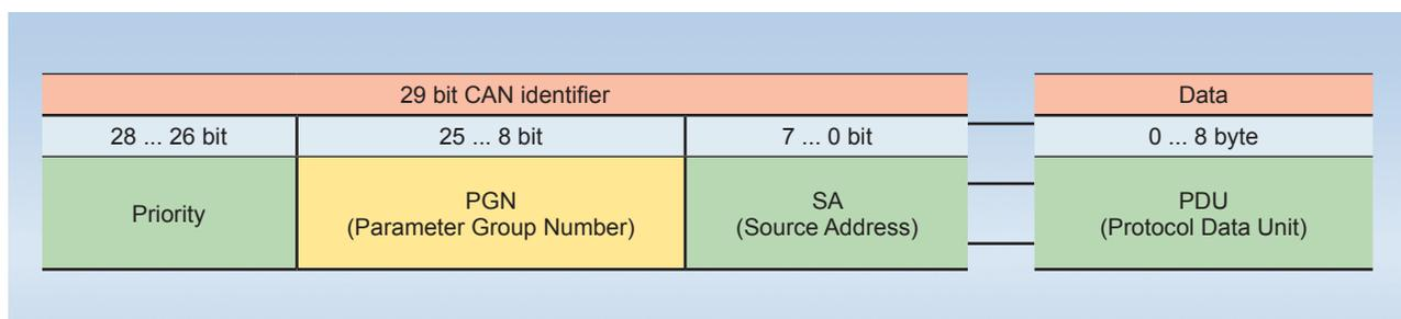
Fig. 15: Data format in the CAN J1939 protocol
