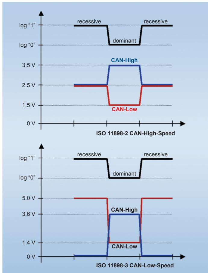
Fig. 2: CAN signal and voltage level
