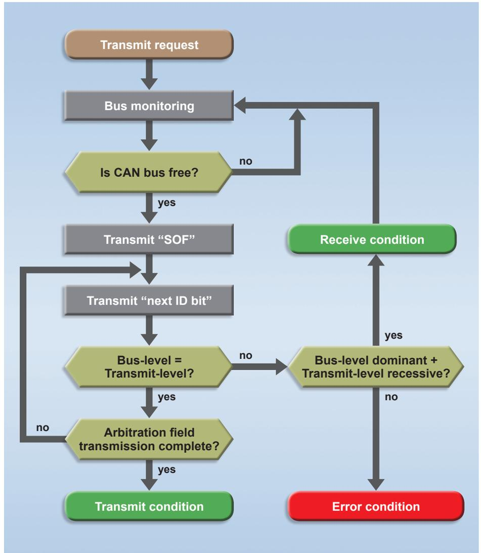
Fig. 14: Bus access using CSMA/CA
