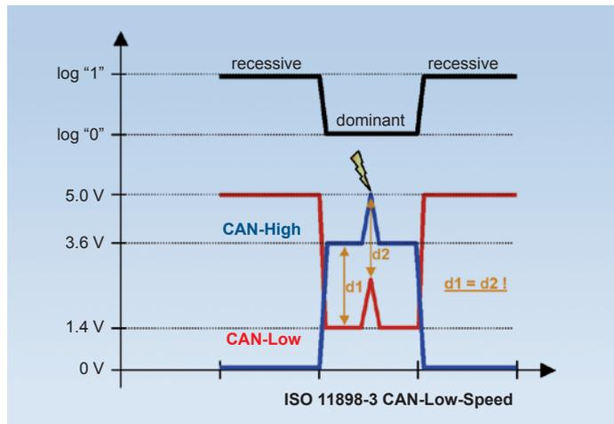
Fig. 3: Electrical interference on CAN bus line
