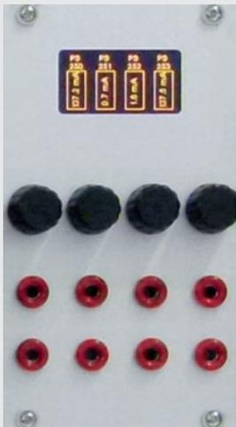
The sensor supply simulation module allows the sensor power supply supplied by the ECU to be tested. It is thus possible to measure the real-time voltage as well as the current. In addition different error signals can be switched.
