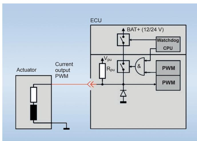
One problem when operating proportional valves with solenoid coils is that the solenoid coil increases its resistance as it heats up. This increase in internal resistance has the effect of reducing the coil current for the same supply voltage. Since the coil current is in turn proportional to the positioning force of the solenoid, the spool position of the valve also changes. To counteract this shift in the hydraulic operating point, the coil current can be measured and thereby also controlled.
