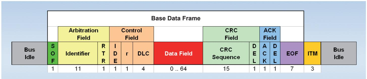
Fig. 9: Format of a CAN Data frame
