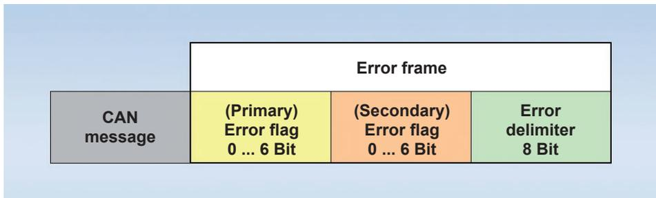
Fig. 12: Format of a CAN Error frame
