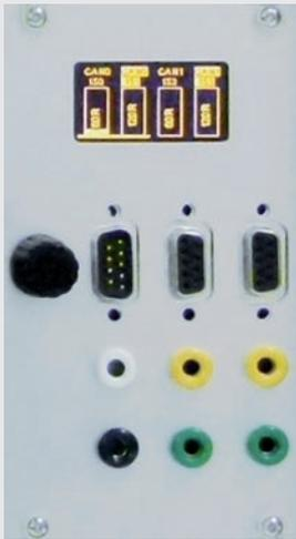
The data interfaces of the connected controller can be tested using the communications module. Specifically using the CAN interface, it is possible to enable termination resistors and to switch short circuits to other states.
