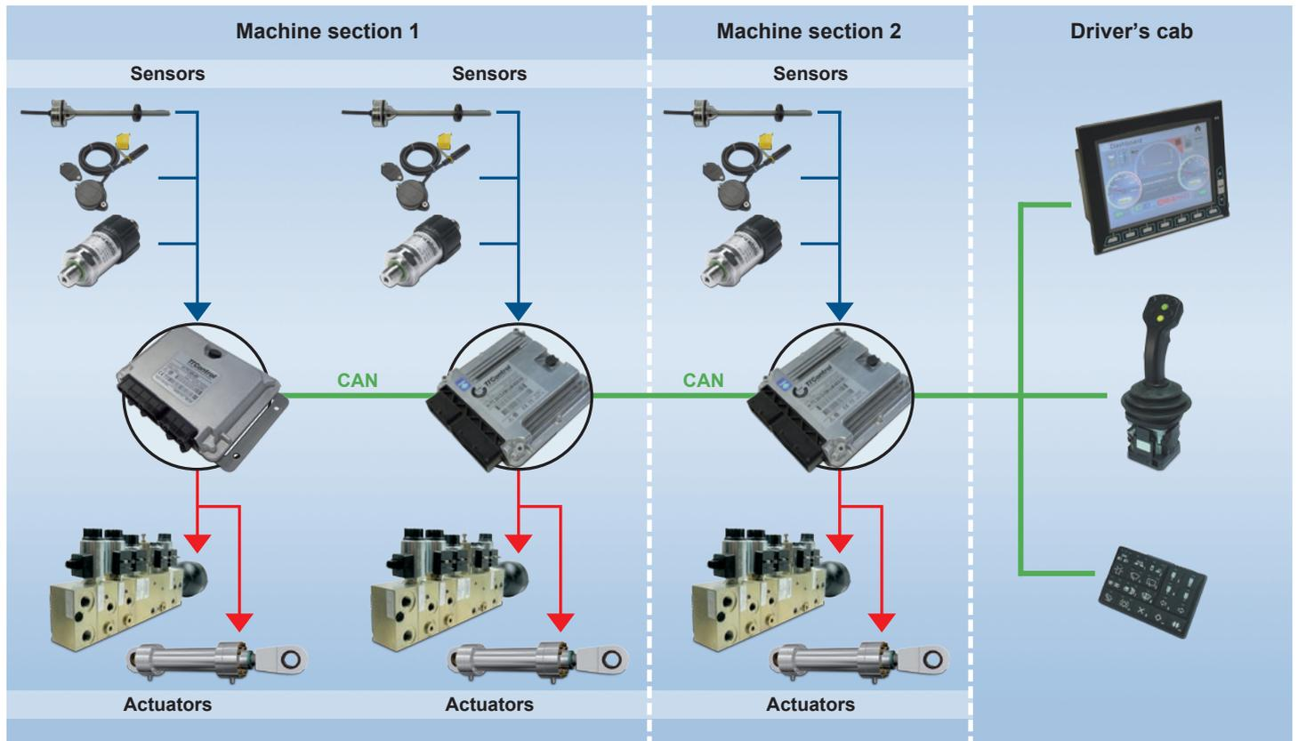
Fig. 21: Decentralized structure with two controllers and an I/O expansion module
