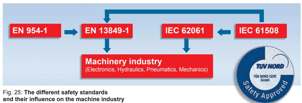
Fig. 25: The different safety standards and their influence on the machine industry
