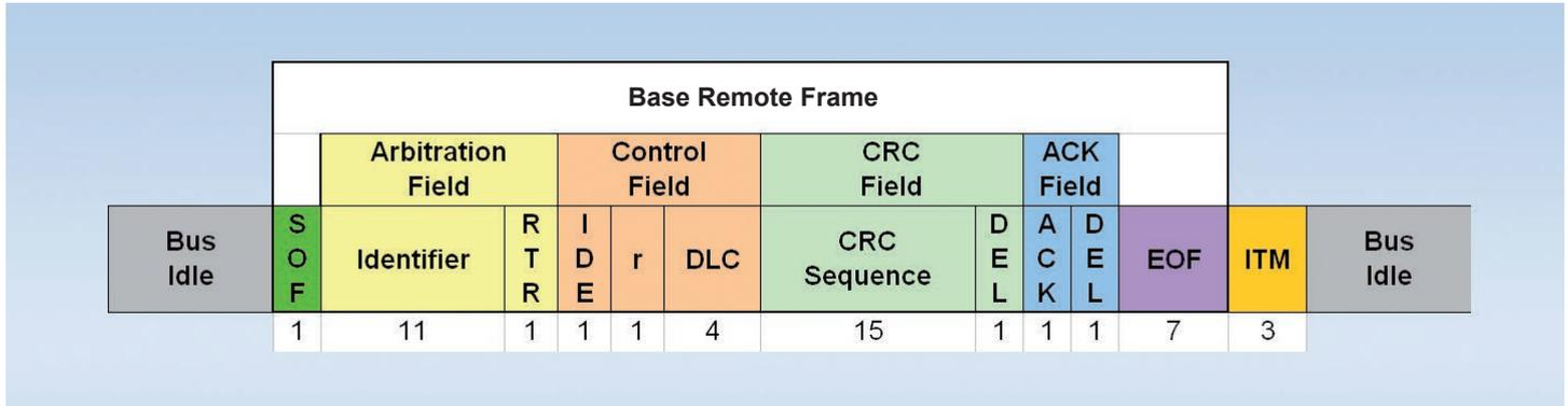
Fig. 11: Format of a CAN Remote frame
