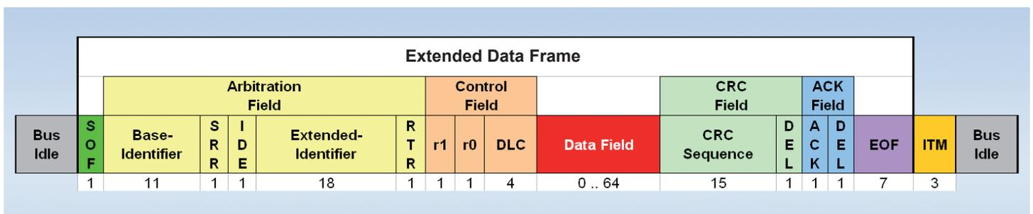
Fig. 10: Format of an extended CAN Data frame
