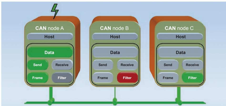
Fig. 7: Schematic of CAN communication (3)
