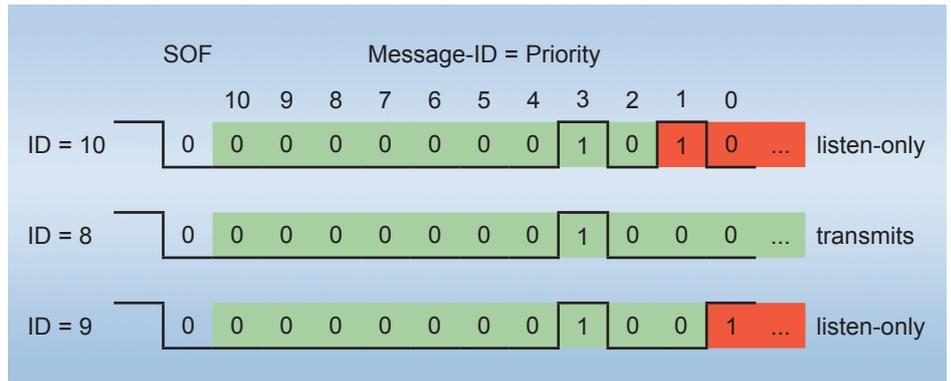
Fig. 13: Arbitration of transmission rights
