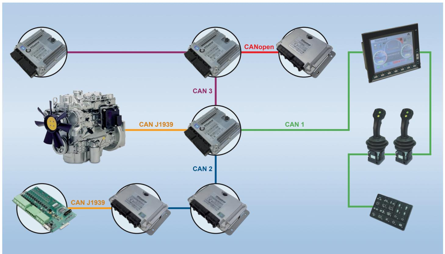
Fig. 22: Decentralized structure with several controllers, I/O expansion modules and sub-networks
