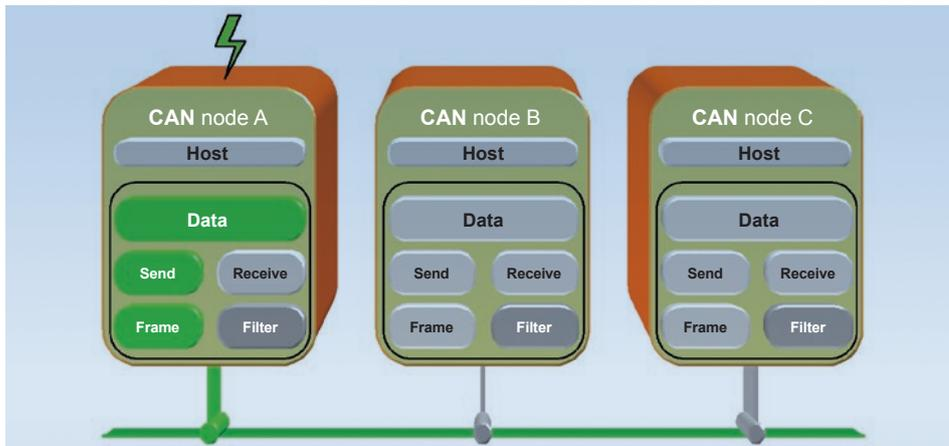
Fig. 6: Schematic of CAN communication (2)
