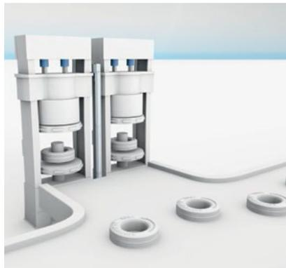
In hydraulic heat presses, green tires receive their correct shape. It is important to achieve consistent quality. Micropulse transducers BTL ensure high repeat accuracy and the exactly identical result at all times. They satisfy the highest requirements of the manufacturing process.
