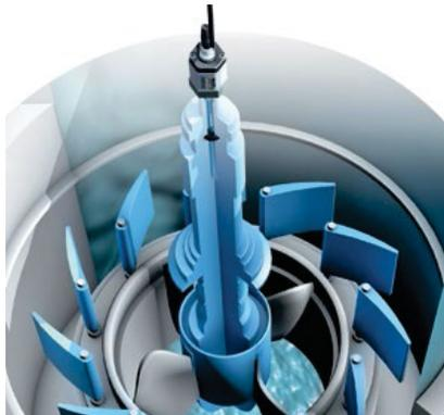
The guide and rotor blades on Kaplan turbines can be adjusted with help from BTL micropulse transducers. For example, a BTL profile controls the position of the guide vanes as needed. Another BTL integrated in the shaft ensures optimal adaptation of the impeller to the water volume.
