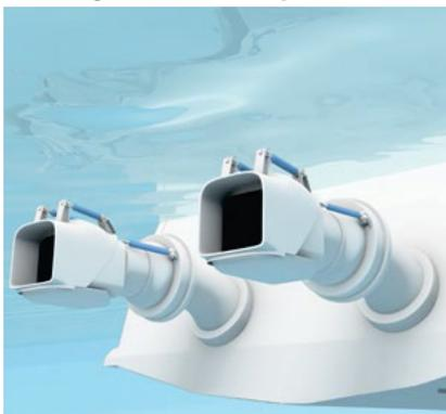
Jet engines are always used if high speeds on the heavy seas or maneuverability in slow travel are required. Hydraulic cylinders move the infeed flap and nozzle to adjust to direction and speed. Micropulse transducers integrated in the cylinders reliably measure movement.
