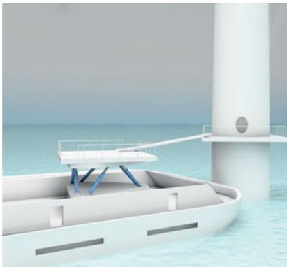
Security on the sea: Even with swelling, people from the supply vessel can safely reach the platform or the offshore wind power plant.
