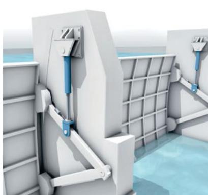
The requirements for a weir go much further than just opening and closing the gate. Fish ladders must be taken into account and the fully automatic control of the water level must be ensured. BSI inclination sensors reliably and precisely measure the intermediate position of the gate.
