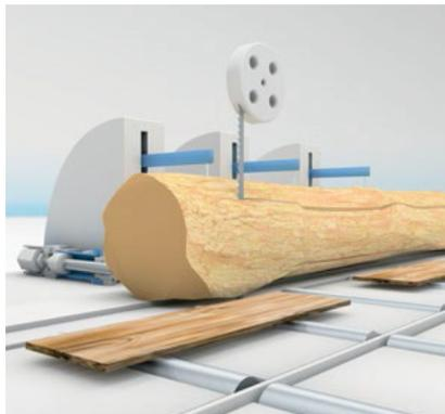
Vertical band saws adjust to maintain the desired board thickness after each cut. Micropulse transducers are excellently suited to configuring these settings quickly and with great versatility.
