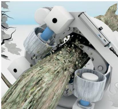
Sensors for debarkers are exposed to strong vibrations. Transducers in hydraulic cylinders monitor the piston position of the infeed unit. This enables logs of different thicknesses to be optimally fed.
