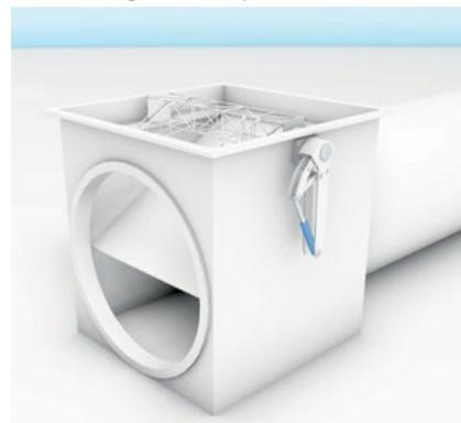
Diverter guide gas turbine fumes. Either to the bypass chimney or to the steam generator. With help from hydraulics and micropulse displacement sensors integrated in them, the diverter can be opened or closed in increments.
