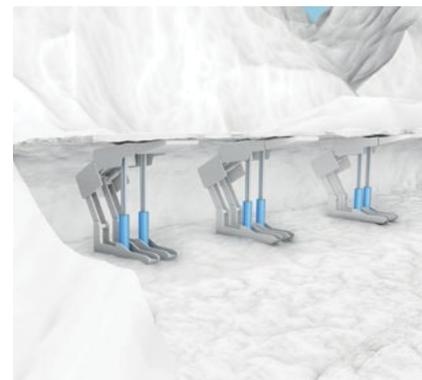
In mining, shields prevent rocks from falling in the working area and injuring miners. To support longwall mining, hydraulic cylinders are used. Micropulse BTL position measurement systems of the K series integrated in the hydraulic cylinders provide exact positioning and secure monitoring of the shields.
