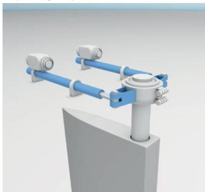
To keep a ship on target, the ship rudder must be continuously adjusted. This is successful with reliable and high-precision Balluff position measurement technology. Position measurement systems BTL rod (integrated in the hydraulic cylinder) and BTL profile check the rudder position from start to finish and allow for exact readjustment.
