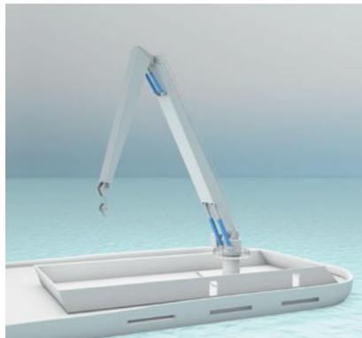
Cranes are used not only in the harbor, but also on the sea. So that safe work is possible, hydraulics and sensors attuned to the harsh sea are needed. Thus, explosion-protected high-pressure resistant inductive sensors reliably measure the end position of the offshore crane, even with high swelling.
