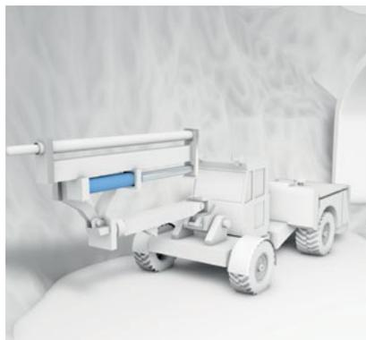
In raw material extraction, Micropulse BTL profile position measurement systems installed outside the cylinders monitor the drilling of the blast holes below ground. This is the only way that safe and reliable tunnel mining and efficient raw material excavation can be ensured.
