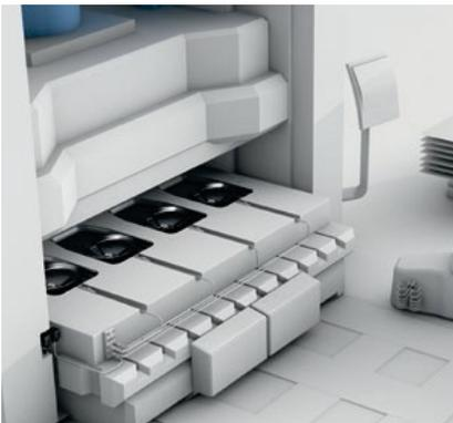
When producing components from carbon-fiber-reinforced plastic (CFRP), the carbon fibers that are woven to mats are pressed into shape under heat and pressure. In this process, they must be monitored and harden uniformly. Micropulse transducers ensure uniform pressure with every press-fitting process without being impeded by heat.
